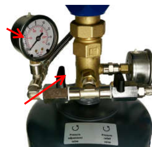
Washing pressure adjustment valve
